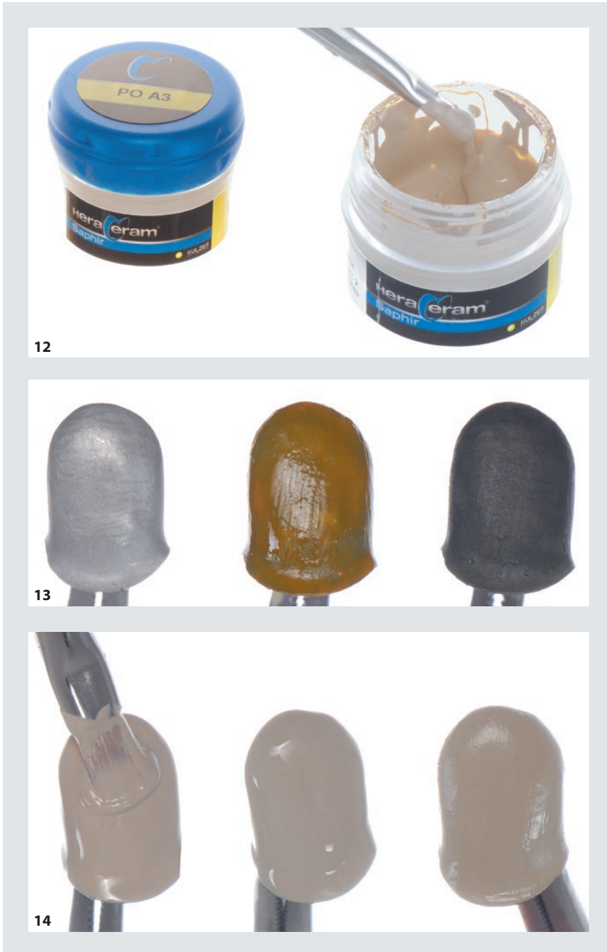
Fig 12 A new generation of paste opaque enables maximum efficiency. Fig 13 The use of HeraCeram NP-Primer makes the oxidation firing unnecessary and prepares the framework surface for the application of the opaque. Fig 14 Thanks to the adhesive force of the newly developed paste opaque, the metal frameworks can be completely masked with a single opaque firing.
