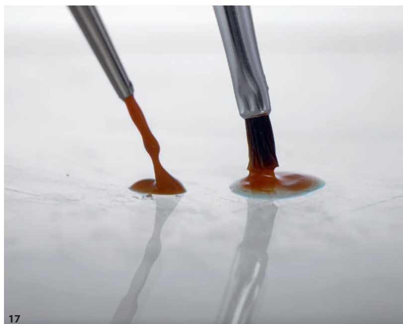
Fig. 14 The enamel is reduced according to the required reference shade or teeth. Fig. 15 The reduced surface is activated with Signum liquid and further processed. Fig. 16 The Signum cre-active stains provide users with a 3D characterisation system. Fig. 17 Thanks to the cre-active transparent materials T1 and T2 the required viscosity can be individually adjusted.
